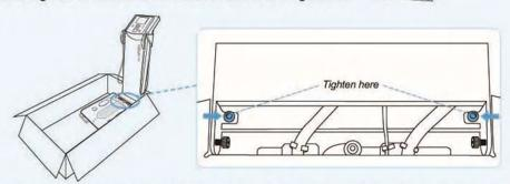
Mold the upper part and center of lower part with two people and take the equipment out of the carton. Place the equipment at desired area and tighten the 4 screws connecting upper and lower parts with a hexagonal wrench.
